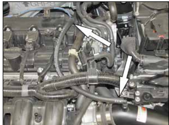
22. Install the provided crank case vent hose onto the valve cover port and then onto the 90° fitting in the intake tube. NOTE: Some trimming of the hose may be necessary.
