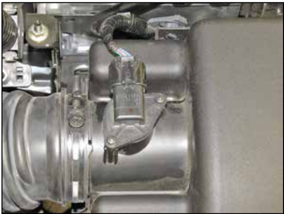
3. Disconnect the mass air sensor electrical connection.
