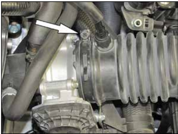
5. Loosen the hose clamp securing the factory intake hose to the throttle body.
