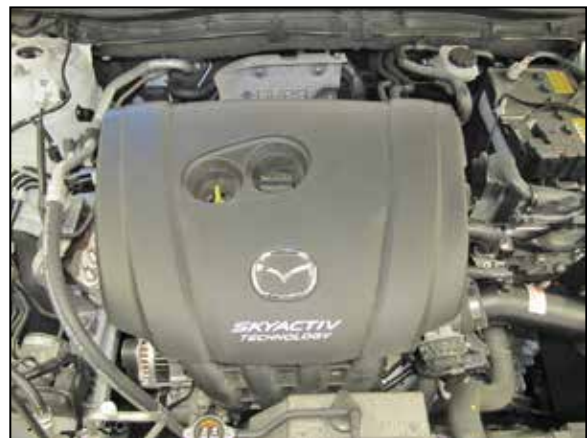
23. Reinstall the engine cover.
